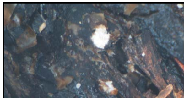
Photomicrograph 1. At 70X magnification, the deposit is revealed as an agglomeration of sand particulates, charred organics, hardness crystals, and other debris.
