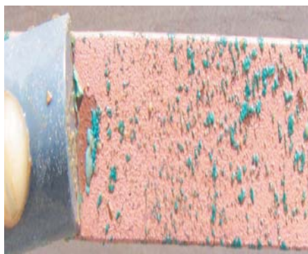
Exposed Corrosion Coupon
